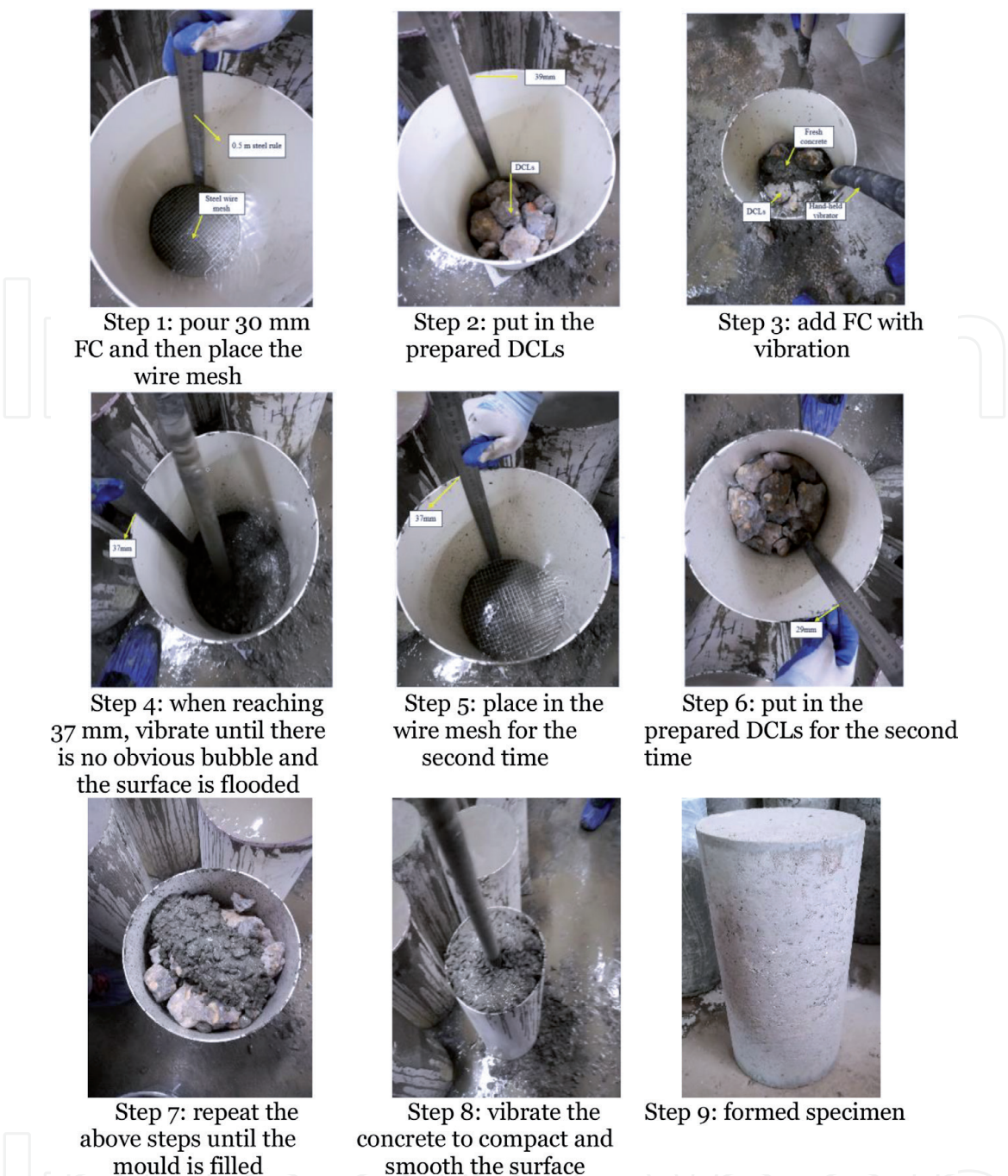
Figure 3. Construction process of specimens.
