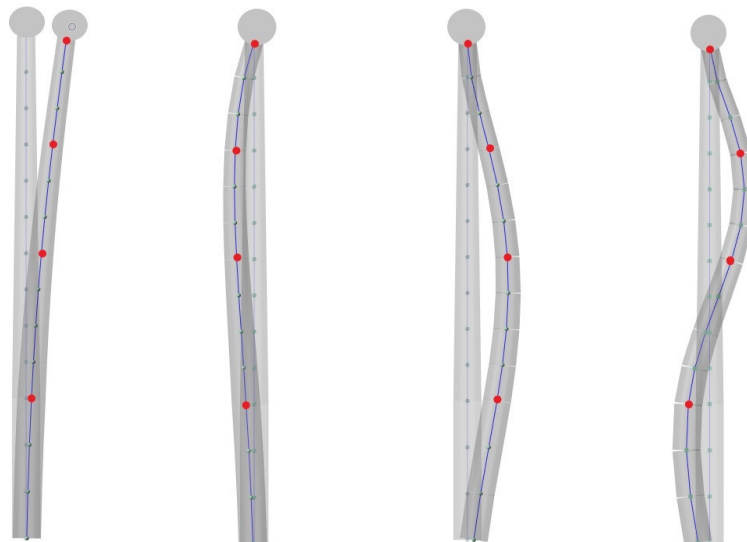
Figure 3.6: Uncoupled tower mode shapes. The first, second, third, and fourth fore-aft mode shapes are shown from left to right respectively. The red points represent Sensor 1, Sensor 2, Sensor 3, Sensor 4, from bottom to top.
