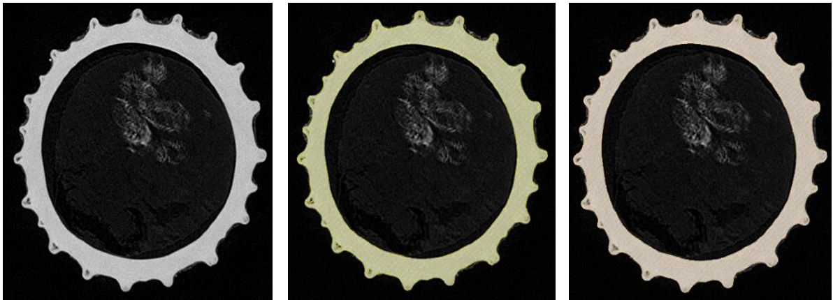
Figure A1. Process of segmentation and reconstruction. Left, scanned specimen. Centre, segmented specimen. Right, reconstructed specimen with holes and dissolve parts cover.
