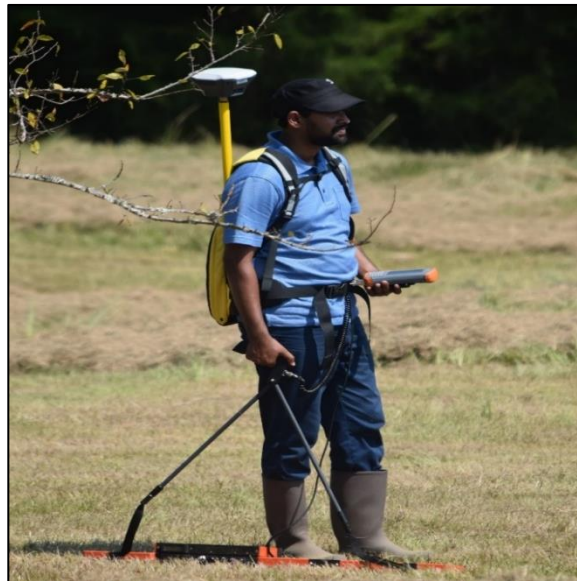
Figure 3.3: EM survey to detect soil collapse features.
