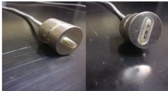
Figure 3.8: Bender element. P source / S receiver (left side), S source / P receiver (right side).
