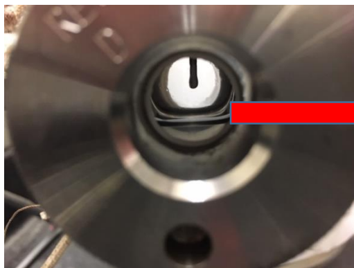
Figure A.6 Cloud point observed at T=41.7\text{ }^{\circ}\text{C} and P=166.03\text{ bar} .
