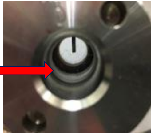
Figure A.2 Cloud point observed at T=50\text{ }^{\circ}\text{C} and P=110.32\text{ bar} .
