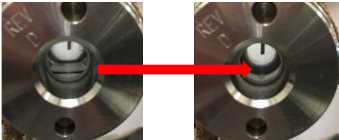
Figure 4.2. Cloud point observed at T=51 °C and P=172.02 bar. Additional images are in Appendix A (p. 78).
