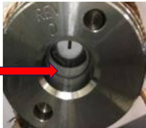
Figure A.3 Cloud point observed at T=60.3\text{ }^{\circ}\text{C} and P=106.87\text{ bar} .
