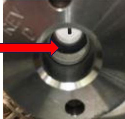
Figure A.1 Cloud point observed at T=40\text{ }^{\circ}\text{C} and P=165.47\text{ bar} .
