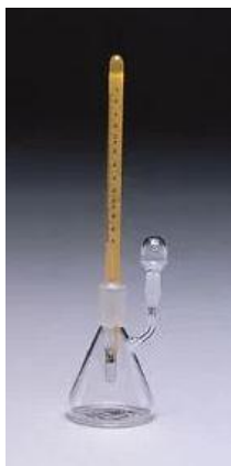
Figure 3.3. Image of pycnometer for measuring wax/n-heptane density.
