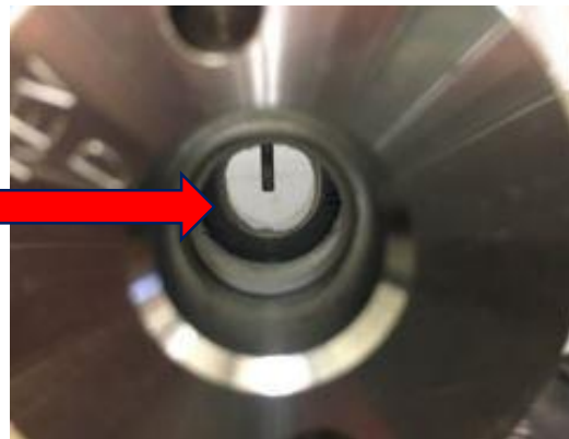
Figure A.4 Cloud point observed at T=57.4\text{ }^{\circ}\text{C} and P=161.89\text{ bar} .
