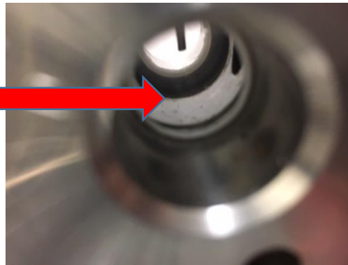
Figure A.7 Cloud point observed at T=49.7\text{ }^{\circ}\text{C} and P=146.86\text{ bar} .
