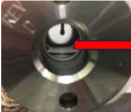
Figure A.1 Cloud point observed at T=40\text{ }^{\circ}\text{C} and P=165.47\text{ bar} .
