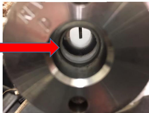
Figure A.6 Cloud point observed at T=41.7\text{ }^{\circ}\text{C} and P=166.03\text{ bar} .
