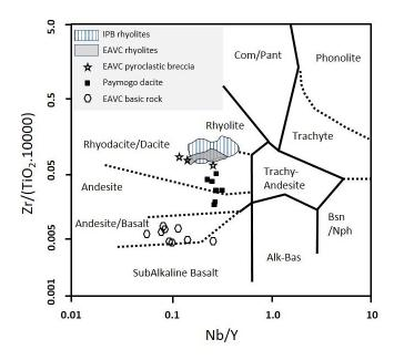
**Figure 5.** Classification of the felsic and mafic rocks in the EAVC area according to the proposal by Winchester and Floyd [51]. Data of "IPB rhyolites" were taken from [12,14]. "Paymogo Dacite" samples were taken from [14].
