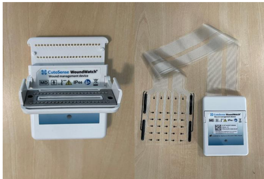
Figure 7. Photograph of the measurement device which is used for the impedance measurement along with the electrode dressing connected to it.
