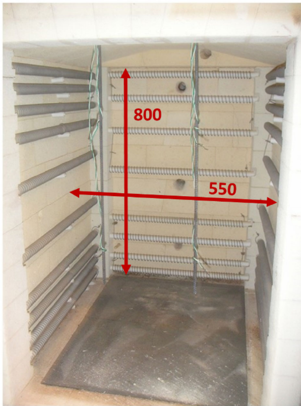
Figure 5. Electric Ceramotherm furnace with inside dimensions of 550 mm × 700 mm × 800 mm.
