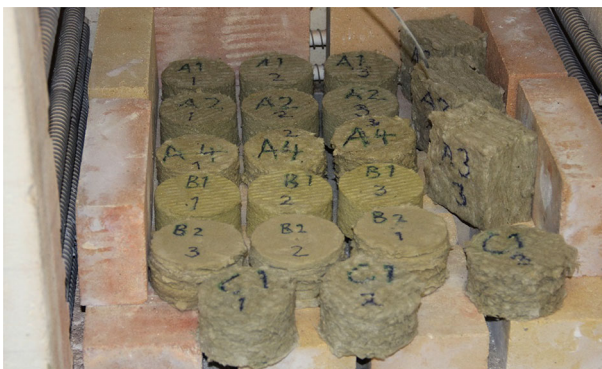
Figure 6. Test samples with a diameter of 90 mm and thickness of 50 mm set in the electric furnace to determine the amount of organic material.
