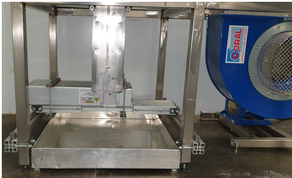
Figure 24. HiWatch HR2 mounted on a track under the wind tunnel. The centrifugal fan can also be seen on the right.
