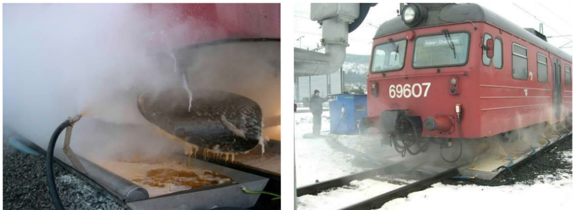
Figure 16. Propylene glycol used for anti-icing. [7]
