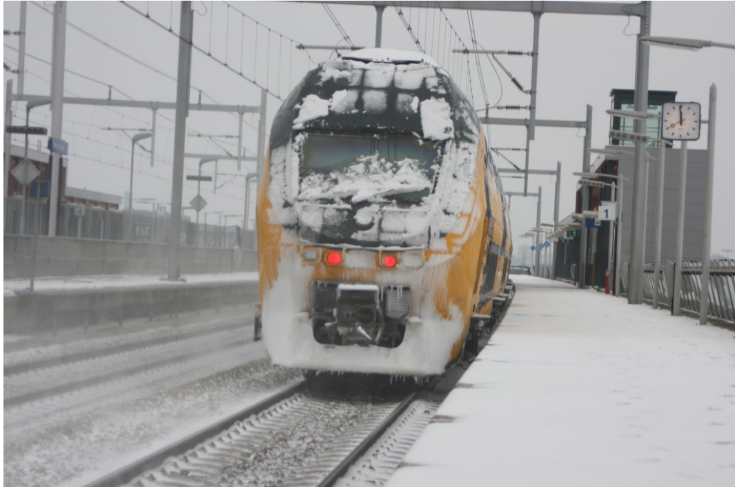
Figure 8. A train engine covered in ice, with the front window frozen over. [42]
