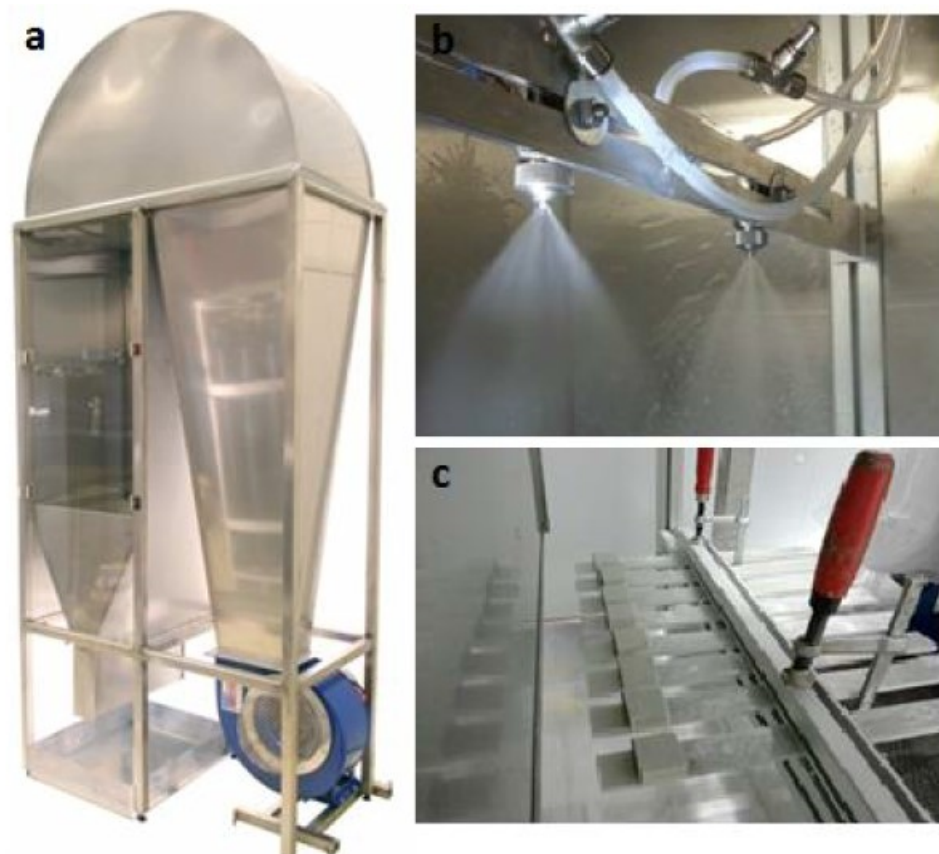
Figure 20. The wind tunnel machinery: a) The complete wind tunnel, b) water and air nozzles inside the tunnel, c) adhesion samples under the tunnel during icing. [44]
