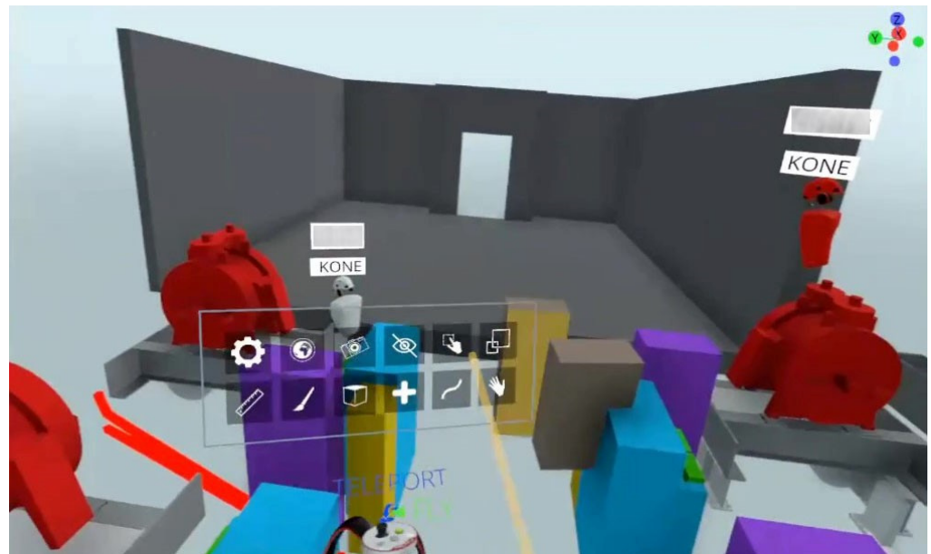
Figure 13. A VR scene of components falling apart due to a synchronization issue, Case 4.
