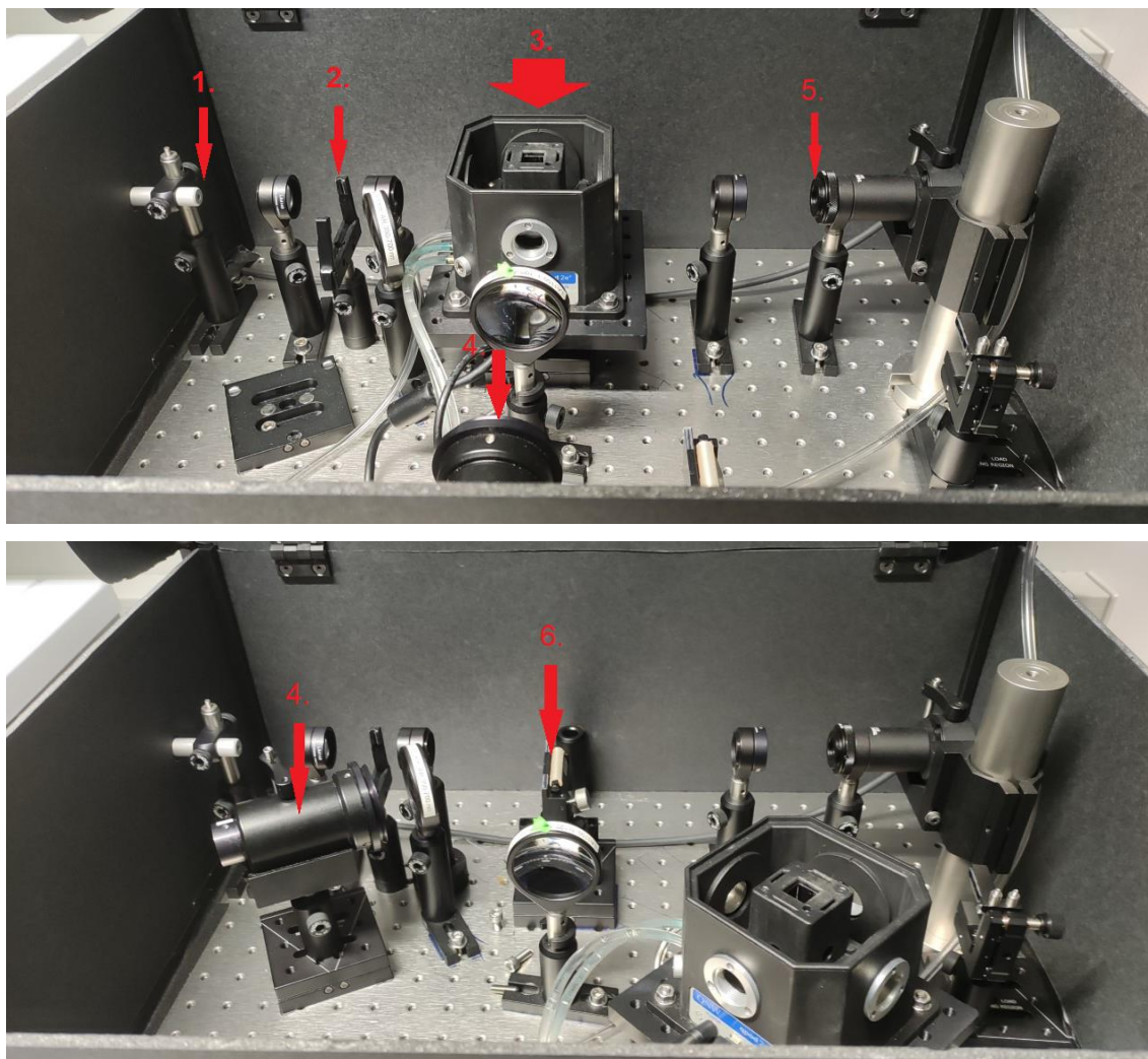
Figure 28 Spectrometer setup built by Dr. Matti Virkki, above for solution measurements and below for solid samples. 1. spectrometer beam in to the setup, 2. holder for polarizer, 3. cuvette holder, 4. LED beam collimator, 5. spectrometer beam back to spectrometer, 6. sample holder.
