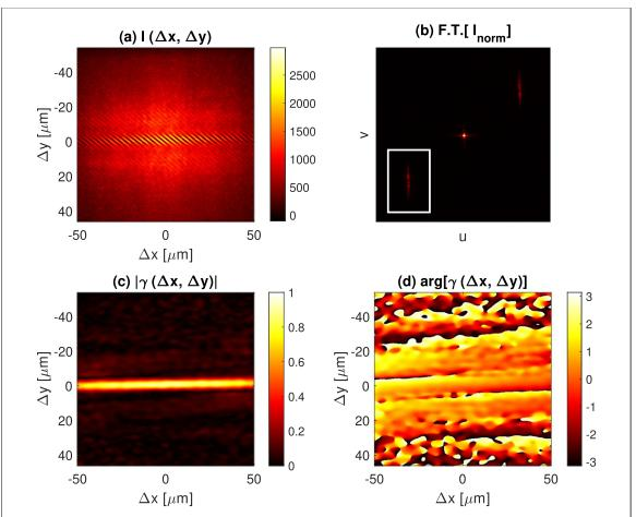
**Figure 5.** WFI measurement of the PLL source pumped with a fluence of 575  $\mu$ J cm<sup>-2</sup>. (a) Interference fringes obtained with both arms open. (b) Fourier transform of the normalized interference pattern. (c) and (d) Are the respective complex degree of spatial coherence and its phase.
