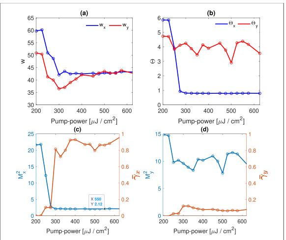
Figure 6. Evolution of the measured beam radii as a function of pump power. (a) The source plane beam widths, and (b) the far-field angular widths of the PLL radiation. (c)  $M_{\chi}^2$ , and (d)  $M_{\chi}^2$  superposed with the effective degree of coherence as a function of pump power. Blue: M2 values, orange: overall degrees of coherence.
