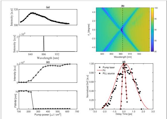
**Figure 2.** (a) Spontaneous emission of dye molecules (top panel) and lasing signal (bottom panel) measured at 180  $\mu$ J cm<sup>-2</sup> and 580  $\mu$ J cm<sup>-2</sup>, respectively. (b) Wavelength and angle resolved transmissivity (%) of the sample. The vertical dash line corresponds to the lasing wavelength. (c) Emission intensity and linewidth as a function of pump power. (d) The normalized autocorrelation for the pump and the PLL pulse.
