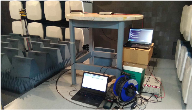
Fig. 4. Anechoic chamber setup for RF WPT experiments.
