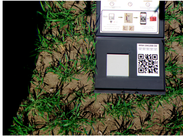
Figure 5. A calibrated reflectance panel (Micasense) placed on the Mustiala biochar field, imaged hand-held using the Micasense Altum multispectral camera.
