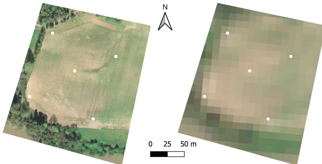
Figure 6. The Mustiala biochar field on 2020-05-22. Left: A 4 cm resolution drone orthomosaic, an artificial view straight down, made of Micasense Altum multispectral camera images without the use of ground control points (GCPs), acquisition time 10:20 to 10:27 (UTC). The geolocation error of GCPs was at most 0.8 m. Right: A 10 m resolution Sentinel-2 satellite bottom-of-atmosphere corrected reflectance image (Copernicus Sentinel Data 2020), acquisition time 09:50 (UTC).
