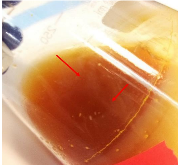
Figure 32. The separate liquid phase on top of the Nessel D100 B 15% of its water solubility medium in experimental day of 2. The separate liquid phase is shown with red arrows.
