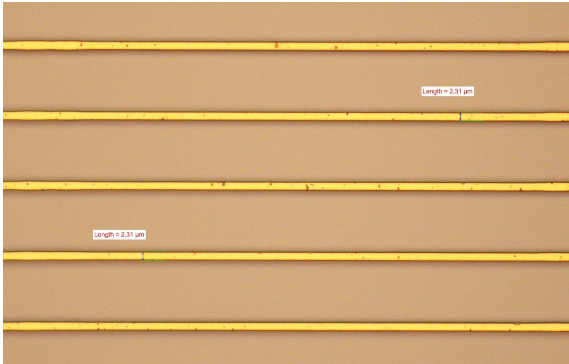
Figure 13. An image of contact fingers taken with the optical microscope with the magnification of 50×.
