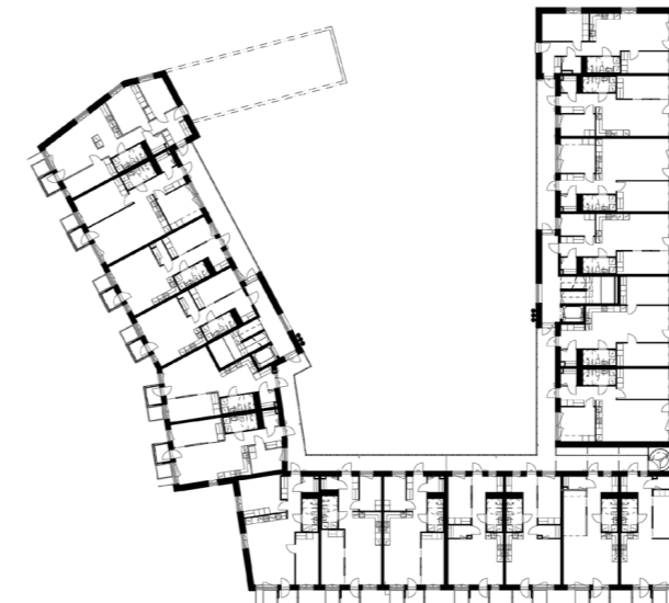
Figure 12. Spatial layout of Vihreistä vihrein provides opportunities for natural ventilation, Talli Architecture & design (Archinfo n.d.)
