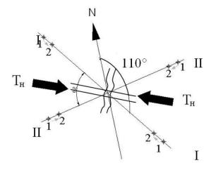
Fig. 8 Schematic of the formation of crossing lines of fault plane with the seam.
