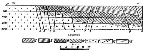
Fig. 2 Schematic geological and structural section of the Western Donbass
