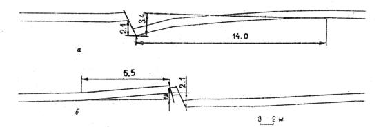
Fig. 10 Seam profile in lava at fault transition: a) at the entrance of lava to the violated zone; b) after moving along the fault plane
