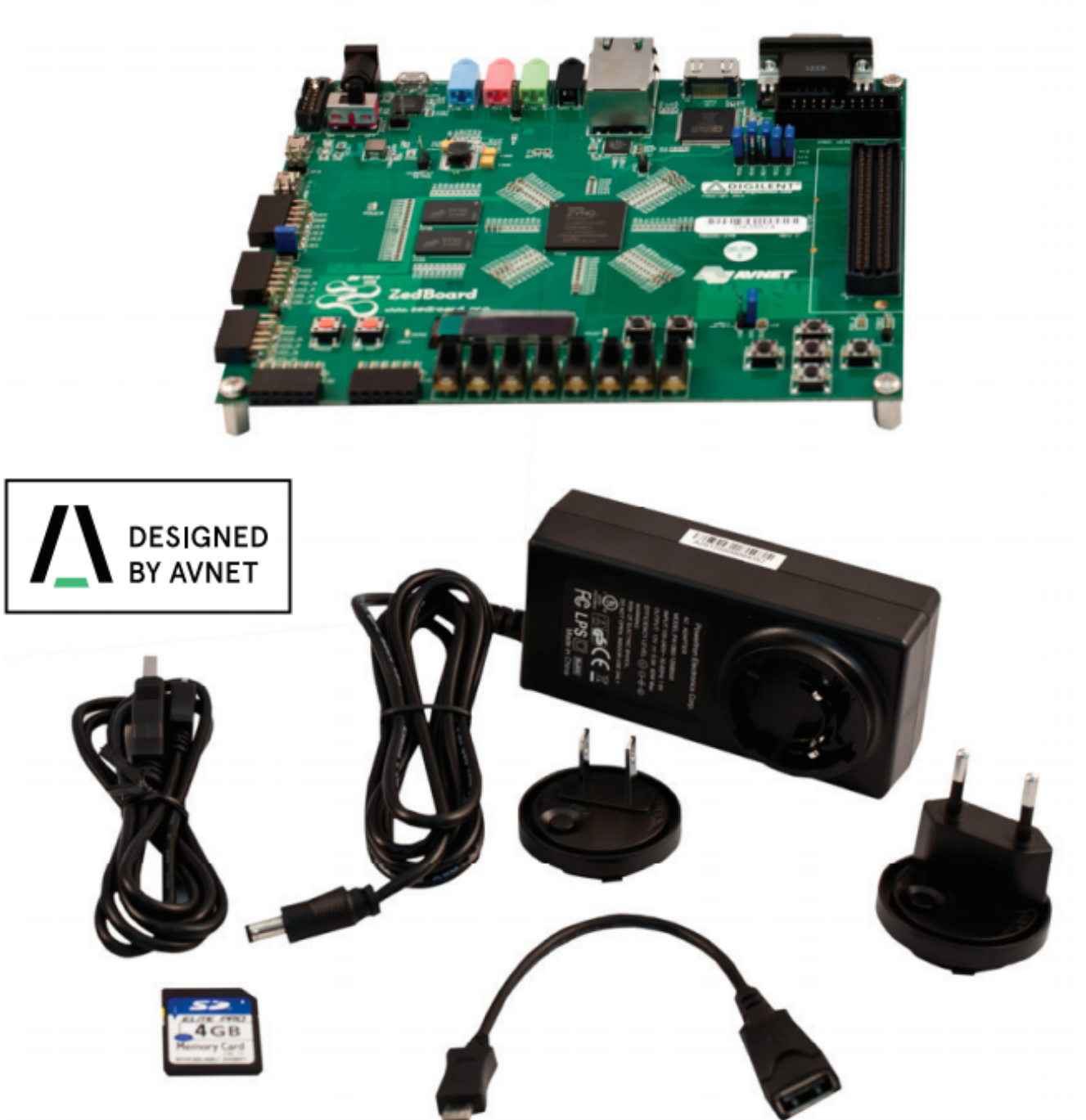
Figure 5: ZedBoard development kit. It includes the Avnet ZedBoard 7020 baseboard, 12 V power supply, 4 GB SD Card, a micro-usb cable, USB adapter (male micro-B to female standard-A).
