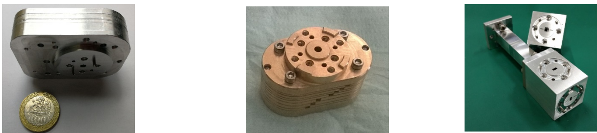
Fig.2. OMT versions of UCh (left panel), INAF (middle panel) and NAOJ (right panel). A 100 Chilean Peso coin (23.5 mm) is shown for scale in the left panel.
