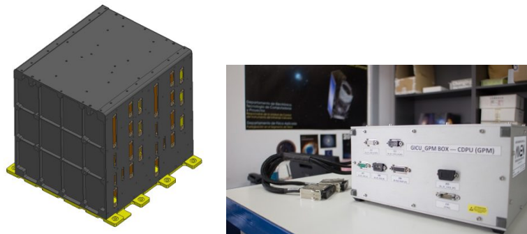
Figure 5-2: NI-ICU mechanical design (left) and EBB of the CDPU board (right).
