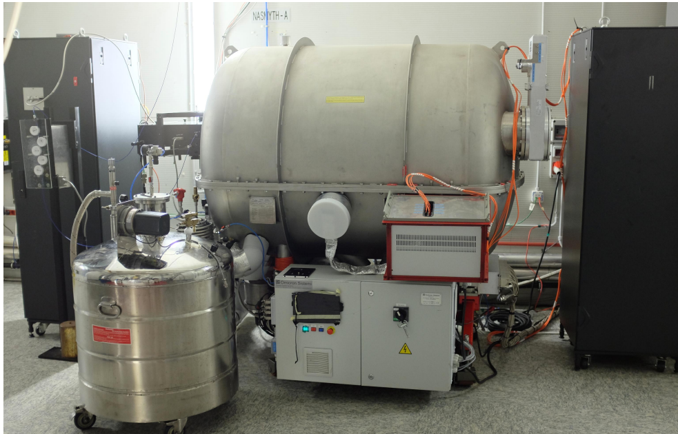
Figure 1: GIANO vacuum vessel, fiber agitator, LN2 tank and the electronics in the Nasmyth-A of TNG.
