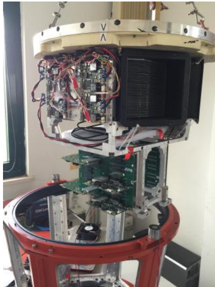
Figure 10 ASTRI-Horn camera at different stages of its assembly. (Top row left) The focal plane and the thermal system are assembled together. Routing of the data and power supply cables is also done. (Top row right) The internal electronics support structure equipped with the BEE, the VDB and the other electronics boards. (Bottom row left) the camera is going to be let into the camera body. (Bottom row right) the ASTRI-Horn camera fully assembled.
