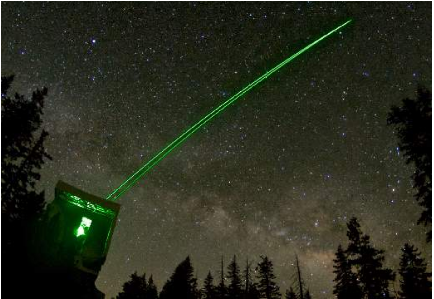
Fig. 1. The ARGOS system propagating a bundle of laser beams on each side of the large binocular telescope. This wide-angle photograph was taken in 2017 with a 25 s exposure time. Each visible green beam in this image consists of three individual laser rays forming the wide-field constellations of guide stars in the atmosphere. The light pulses from the high-power lasers are subject to Rayleigh scattering by air molecules in the Earth’s atmosphere. Having the wavefront sensors gated and adjusted to receive the photons only from a distance of 12 km, a sharp reference beacon constellation is formed. Measuring the wavefronts and correcting the atmospheric ground-layer distortions with the two adaptive secondary mirrors yields a wide-field correction for imaging and spectroscopy.
