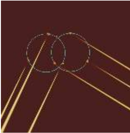
Fig. 6. Image of the double laser constellation on sky, taken with a small auxiliary telescope. Each bundle of lasers belongs to one side of the binocular telescope. The circles guide the eye, showing the constellation diameters of 4 arcmin on sky. The stars indicate the locations of the Rayleigh tip from where the scattered light is used for the wavefront sensing.
