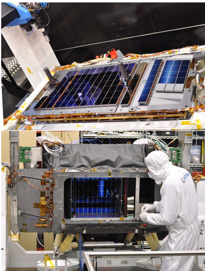
Fig. 5. (Top) Gaia focal plane during assembly. The 14 SkyMapper CCDs are the first two full vertical strips on the left of the SiC structure and the 12 RVS CCDs on the right (the fifth row of white rectangles are not CCDs but are used in thermal control). (Bottom) The integrated focal plane showing the baffles and radiator (extended structure on each side). Again, the RVS CCDs are on the right.
