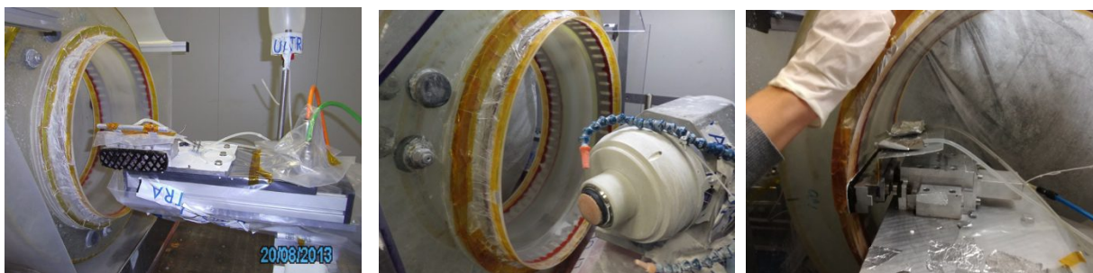
Figure 14: (Left) The polishing phase with a pitch tool. The shell is mounted on the lathe with the optical axis in horizontal position. A liner carriage drives the oscillations of the pitch tool along the optical axis. \text{CeO}_2 slurry is distributed. (Center) The lathe is equipped with a bonnet tool. The \text{CeO}_2 is dispensed through the nozzle, reproducing the nominal Zeeko set-up. (Right) A new polishing set-up is tested on the shell. A layer of TRizact 3M covers the pitch tool. Demineralized water is used instead of slurry.
