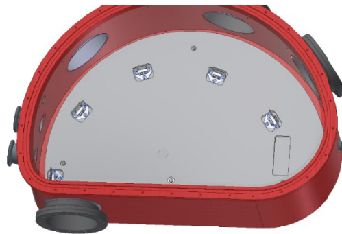
Figure 13: optical bench with the flexures and the central pivot.
