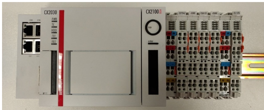
Figure 2. Beckhoff PLC and I/O modules used in the test bench.
