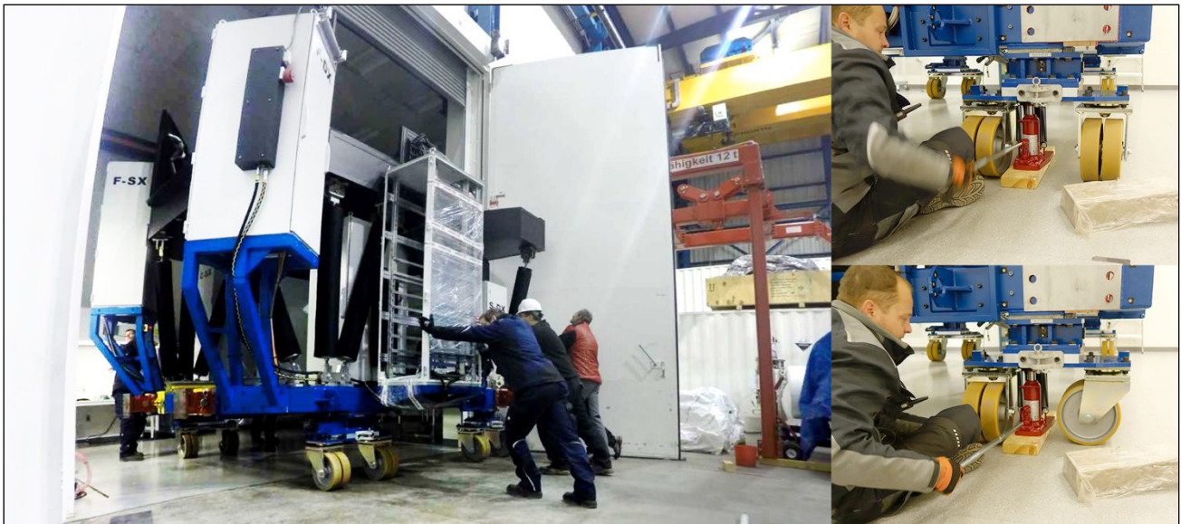
Figure 3. Dealing with instrument size and weight. At almost 10 metric tonnes, LN is no light-weight, but a set of custom wheels permits handling with no motorized aid (left panel). Jacking up the corners of the instrument one at a time and rotating the assemblies 90° lets LN go around corners with zero turning radius (right panels).
