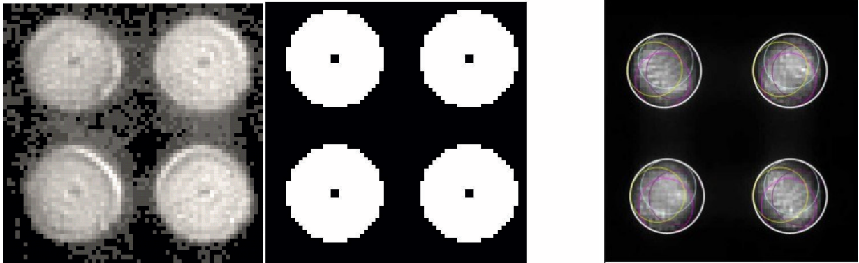
Figure 5. On the left, a frame from the the CCD50 on the GWS WFS looking on a single fiber with AdSec applying the flat shape. On the central panel: the pupil mask as encoded in the Real Time Computer (RTC) software. Here the system used a 2 \times 2 binning on chip, the same used for on sky operations in the case of bright reference stars. On the right the CCD39 is focused in order to make the super imposition of the pupil covering the metapupil (or the Xinetics DM).
