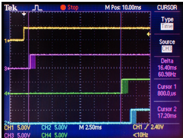
Figure 5: Shutter open signals jitter and timings.
