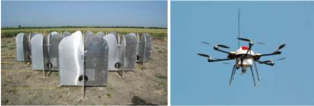
Fig. 5. Picture of MAD array (left) and the UAV equipped with RF transmitter and dipole antenna (right).
