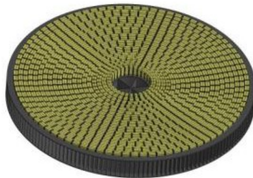
Figure 2. A pictorial view of the 3 m ATHENA optics with the arrangement of the single mirror modules shown.
