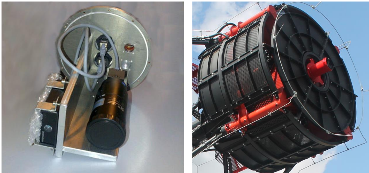
Figure 7: (left) The Pointing Monitor Camera during the integration phase. The PMC support hosts also the sky quality meter (right) The PMC mounted on the support of the secondary mirror of the ASTRI SST-2M telescope prototype.
