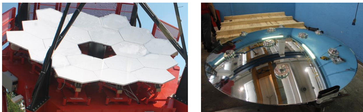
Figure 3: (left) Primary mirror of the ASTRI SST-2M prototype, a plastic film protects the mirrors. (right) The secondary mirror of the ASTRI SST-2M prototype with interfaces seen from its rear side.
