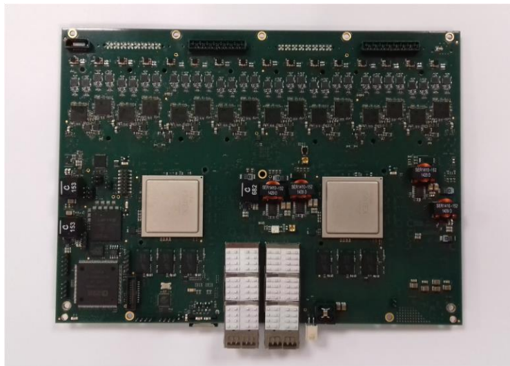
Fig. 3. Analog Digital Unit (ADU) Board includes an analog part, performing high frequency acquisition and conversion of the antennas' RF signals, and a digital part, accomplishing high performance filtering and pre-processing of the acquired data.
