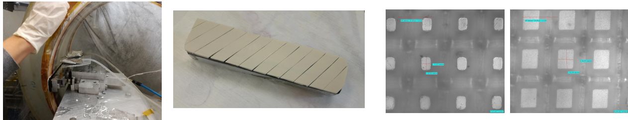
Figure 17: (A) The pitch tool operating on a section of the shell#4. (B) The tool structure with the 3M™ Trizact™ 568XA fixed on the pitch. (C) The 3M™ Trizact™ 568XA pyramids size evolution during the time.
