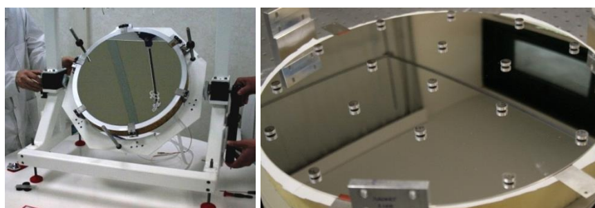
Fig. 1 Left: the OBB assembly on its integration stand. Middle: the back surface of the TS with the 19 magnets.
