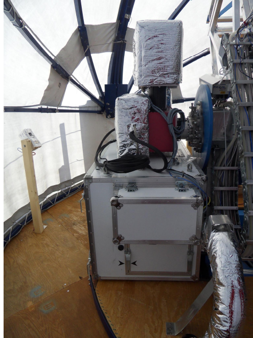
Figure 2 –AMICA mounted at the Nasmyth A focus of ITM. The cryostat (red box) is kept outdoor in such a way the thermal input is extremely reduced and the benefits of the Antarctic environment for infrared observation are fully exploited. All other sensitive devices are hosted inside thermally insulated and controlled racks: a main rack (the white box at the bottom) hosting all the control subsystems, plus three small boxes (covered with a reflecting thermal insulator in the figure) hosting the cold-head, the cryostat vacuum valve and the proximity modules of the readout electronics system.
