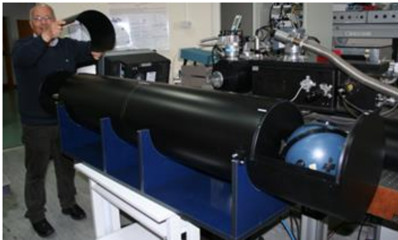
3 Figure 9. Experimental set-up for the angle of incidence measurements. In the upper panel, a 3D view of the system: 1. the tube; 2. source and integrat- 4 ing sphere; 3. the PSAU-CAEN system. In the lower panel, photograph of the actual system.
