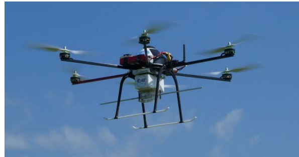
Figure 1: UAV-based flying test source. The payload consists of a GNSS receiver, an RF generator and a dipole antenna.
