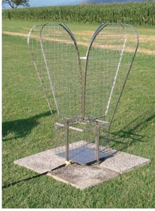
Figure 2: Dual-polarized cavity-backed Vivaldi for the Sardinia Array Demonstrator (SAD). The surface is made of a stainless steel wire mesh.
