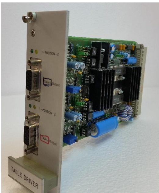
Fig. 2.4.2 a) Table driver developed by IRAM for the receiver calibration system, b) 3D rendering of the control board of the calibration motors we developed for SRT.
