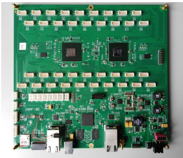
Figure 7. Left : The Back End Electronics. The board dimensions are 220mm x 250mm. Right : Block diagram of the BEE showing the architecture designed for ASTRI SST-2M as implemented inside the Zynq FPGA. The ancillary subsystems controlled by the BEE are also highlighted. On the left, there are the signals that interface each PDM. On the right, there are the LAN links that allows the communication to the external world: the Camera Control and the Camera Server.
