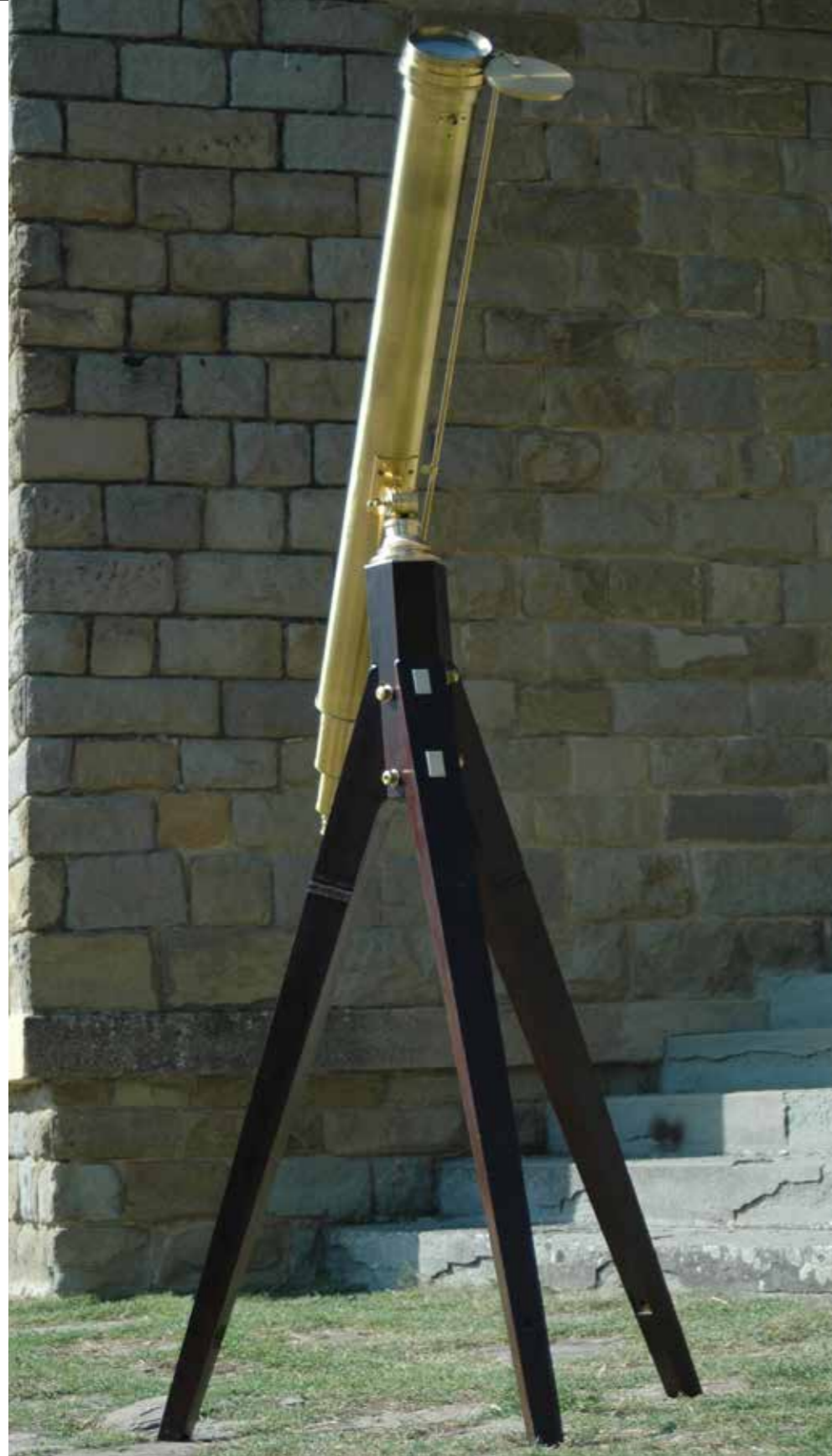
FI. 09. REFRACTING TELESCOPE Steinheil (obiettivo), Munich 1858 brass, wood, glass (obiettivo: 108 mm diameter, 1620 mm focal distance) INAF-Arcetri Astrophysical Observatory, inv. Coll. Scient. e Museali n. 107005001
