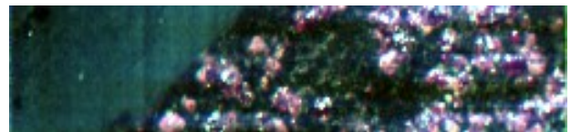
Fig.1. RGB image acquired with SPIM on the thin section (R:0.70 \mu\text{m} , G:0.53 \mu\text{m} , B:0.44 \mu\text{m} ).
