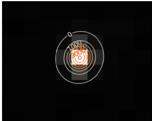
Figure 13 Best focus for the first light acquired during the first commissioning gives PSF FWHM of about 1.2 px
