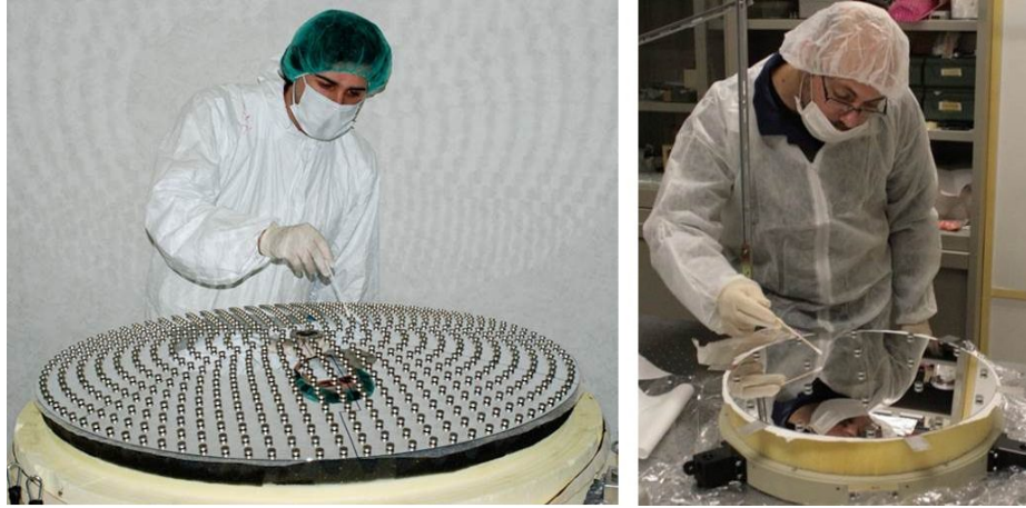
Figure 1. Comparison between the 91 cm LBT TS equipped with 672 magnets (on the left) with the LATT-OBB one (on the right).
