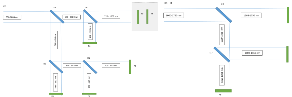
(a) Schematic division of the visible arm. (b) Schematic division of the infrared arm. Figure 6: Schematic division of the optical path of the multiband camera
