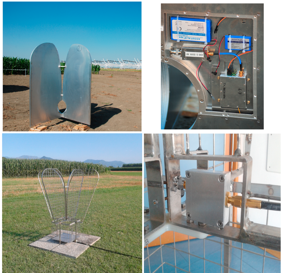
Figure 3. (left column) Antenna mechanics and (right column) zoom for the electronics integration. (top row) Vivaldi 2.0 for MAD; (bottom row) Vivaldi 3.1 for SAD.
