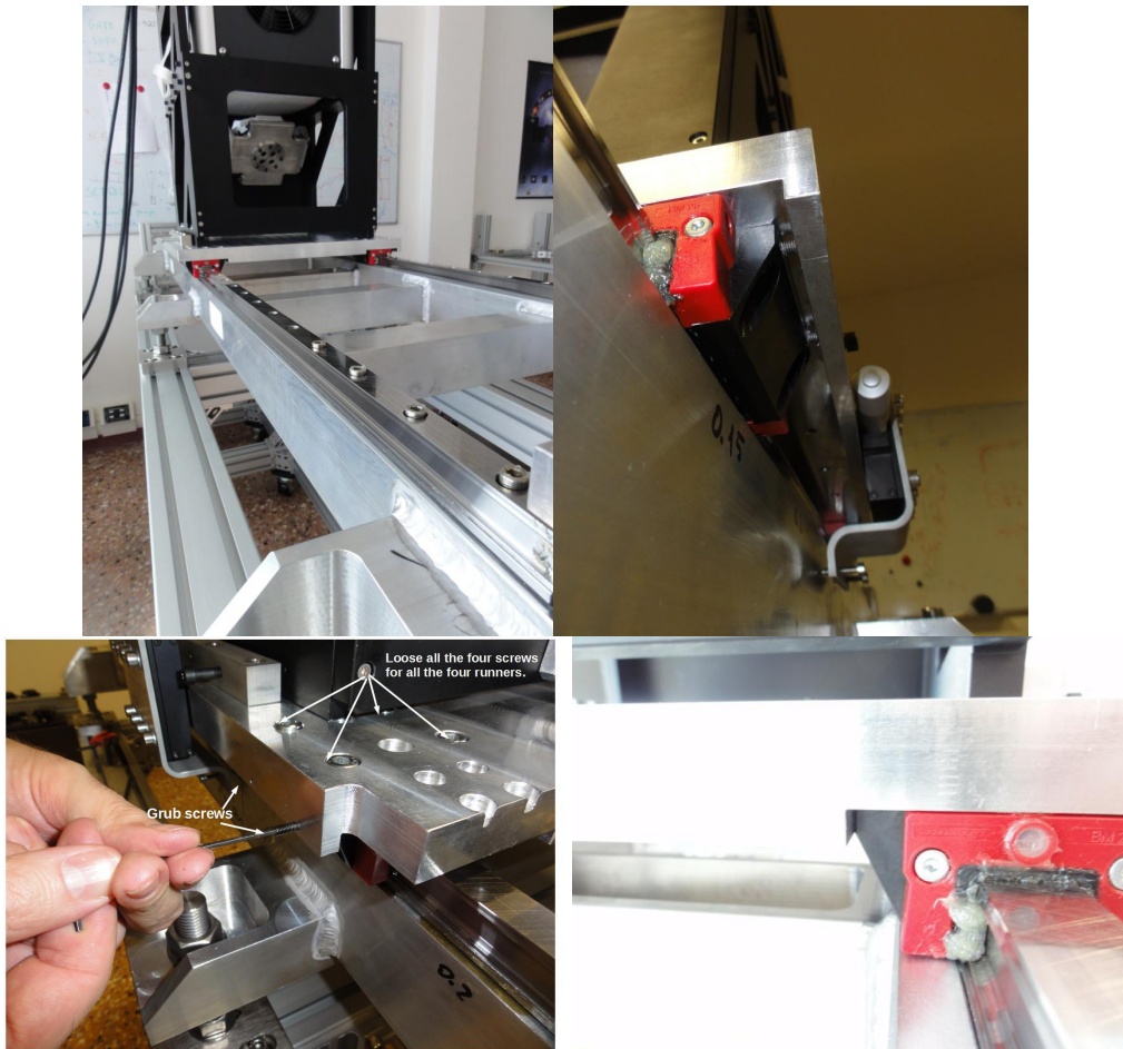
Figure 4 The backlash between the runners on the right rail and the carriage was removed by grub screws. Then, the left rail was aligned by tighten up its screws as they were overtaken by the carriage sliding along its stroke (bottom-right).
